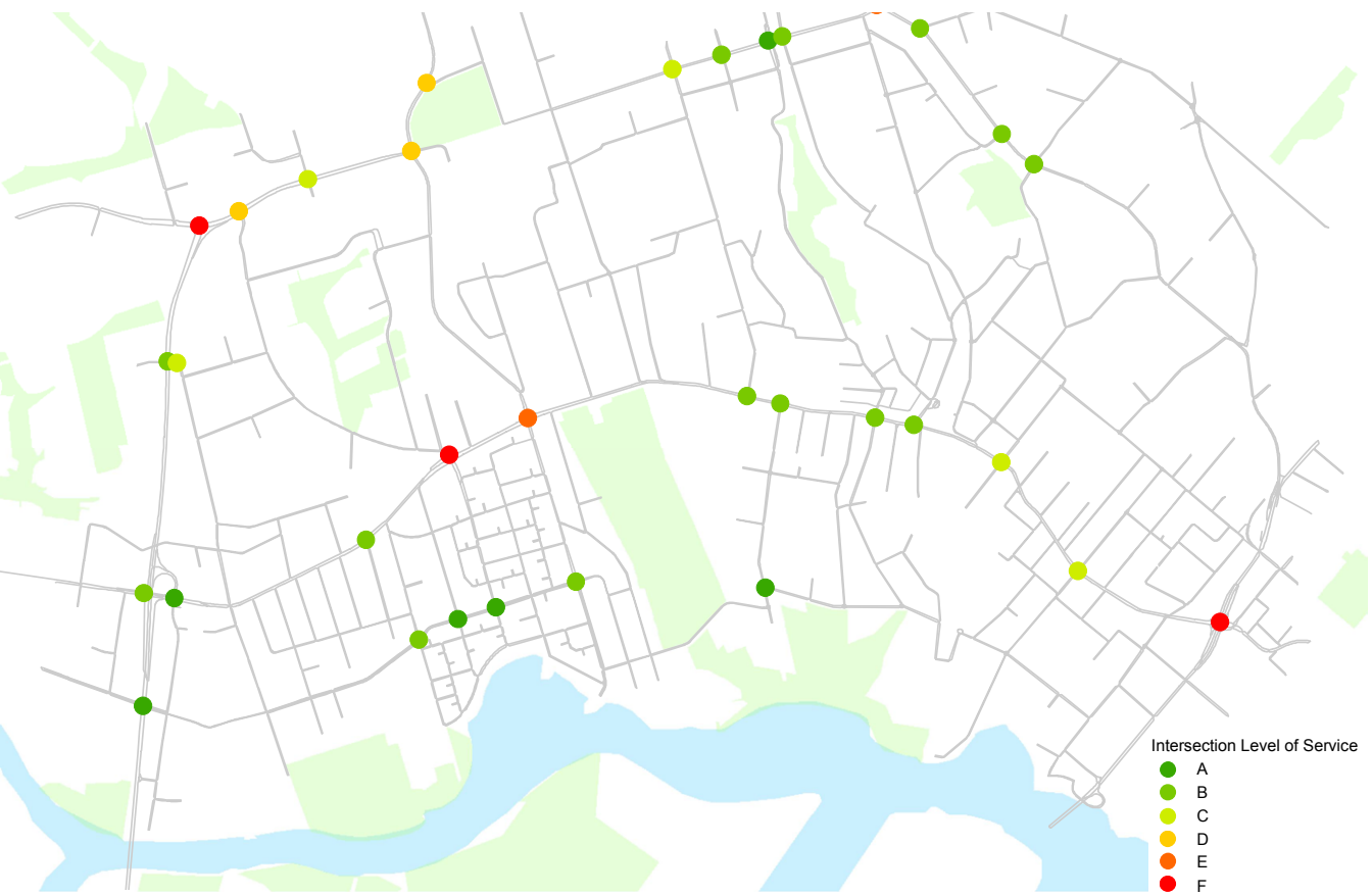
Figure 6.11 : Intersection level of service - 2036 AM with development
