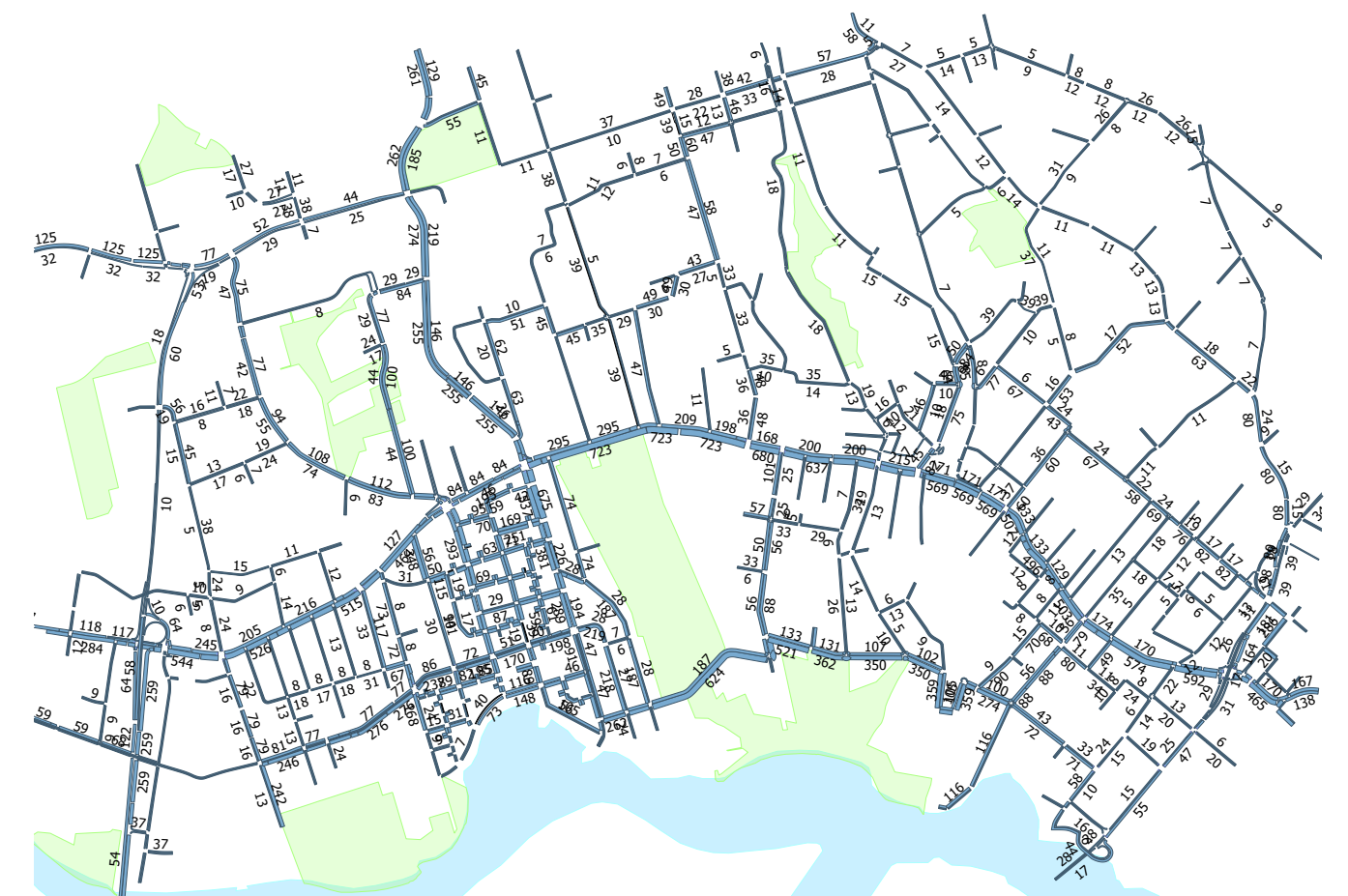
Figure 5.10 Traffic volume - 2036 PM peak hour (only trips generated by development)
