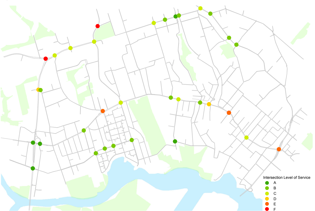
Figure 6.13 : Intersection level of service - 2036 PM with development
