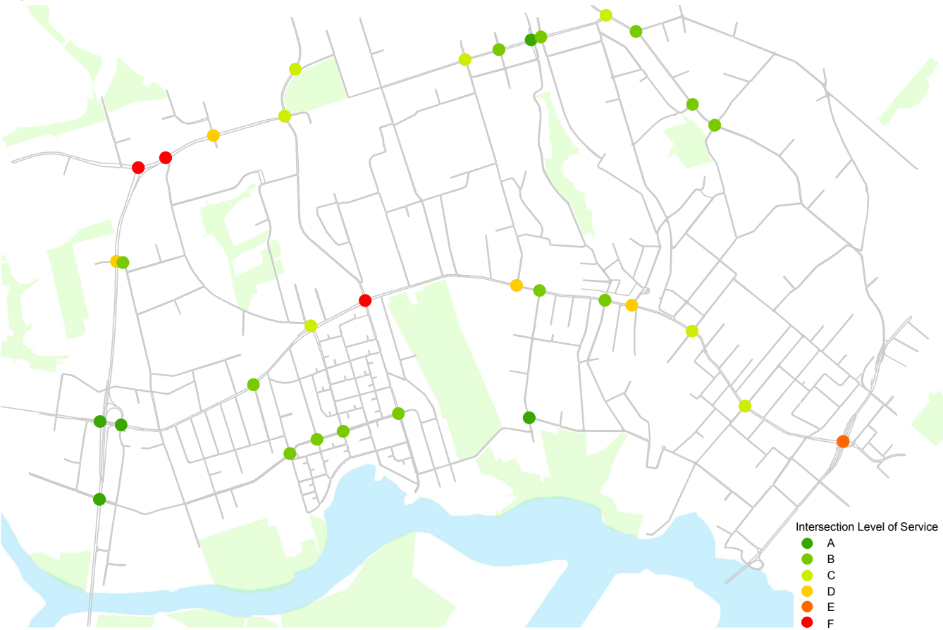
Figure 6.12 : Intersection level of service - 2036 PM do minimum - no development
