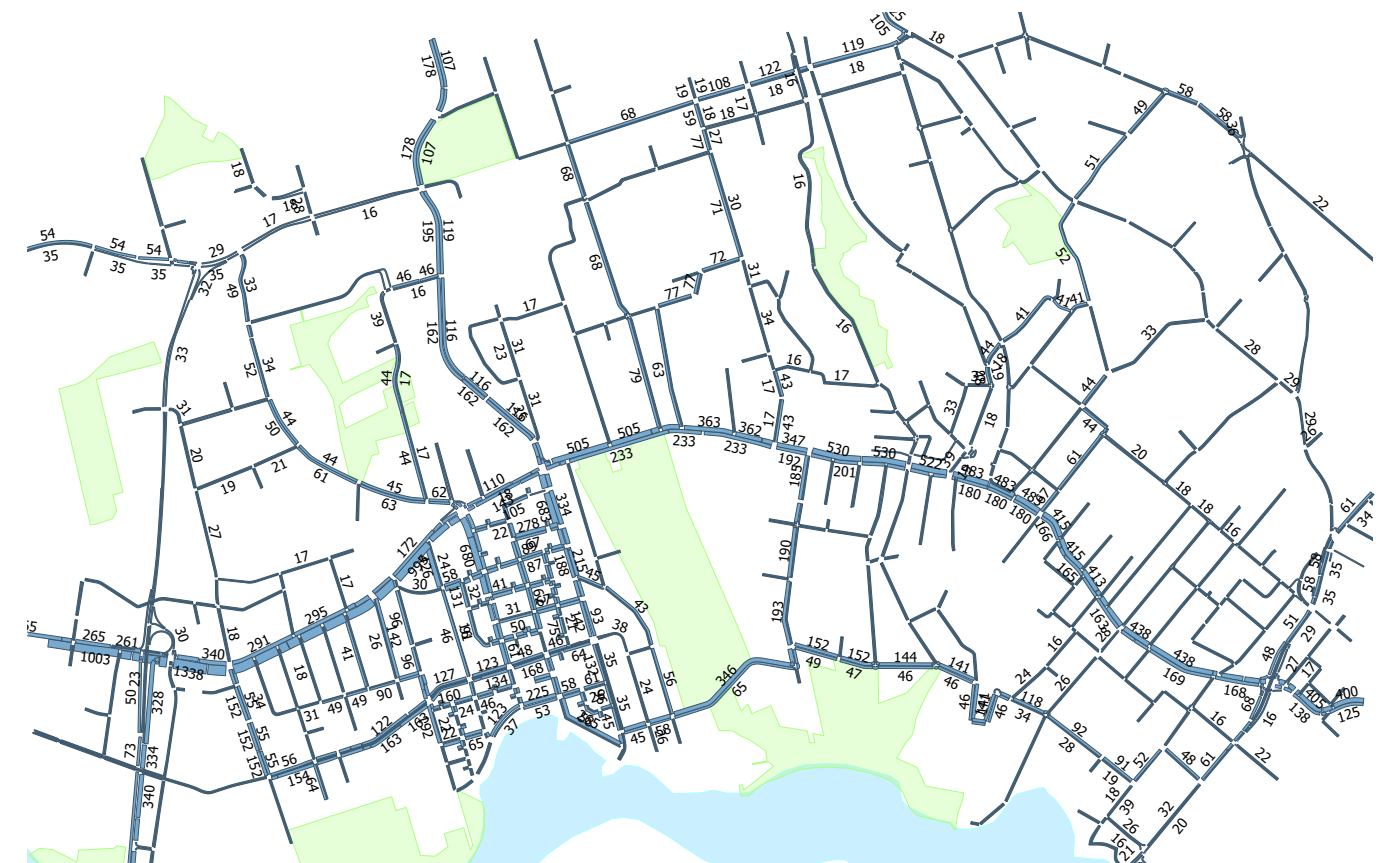
Figure 5.10 Traffic volume - 2036 PM peak hour (only trips generated by development)
